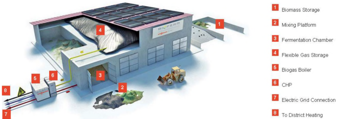
Figure 4: Example of Garage Style Dry Anaerobic Digestion
